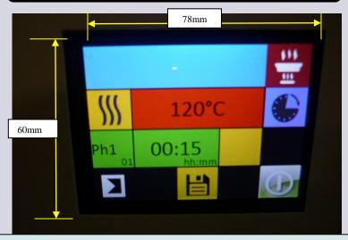
Heating process settings window for liquid heating mode.
